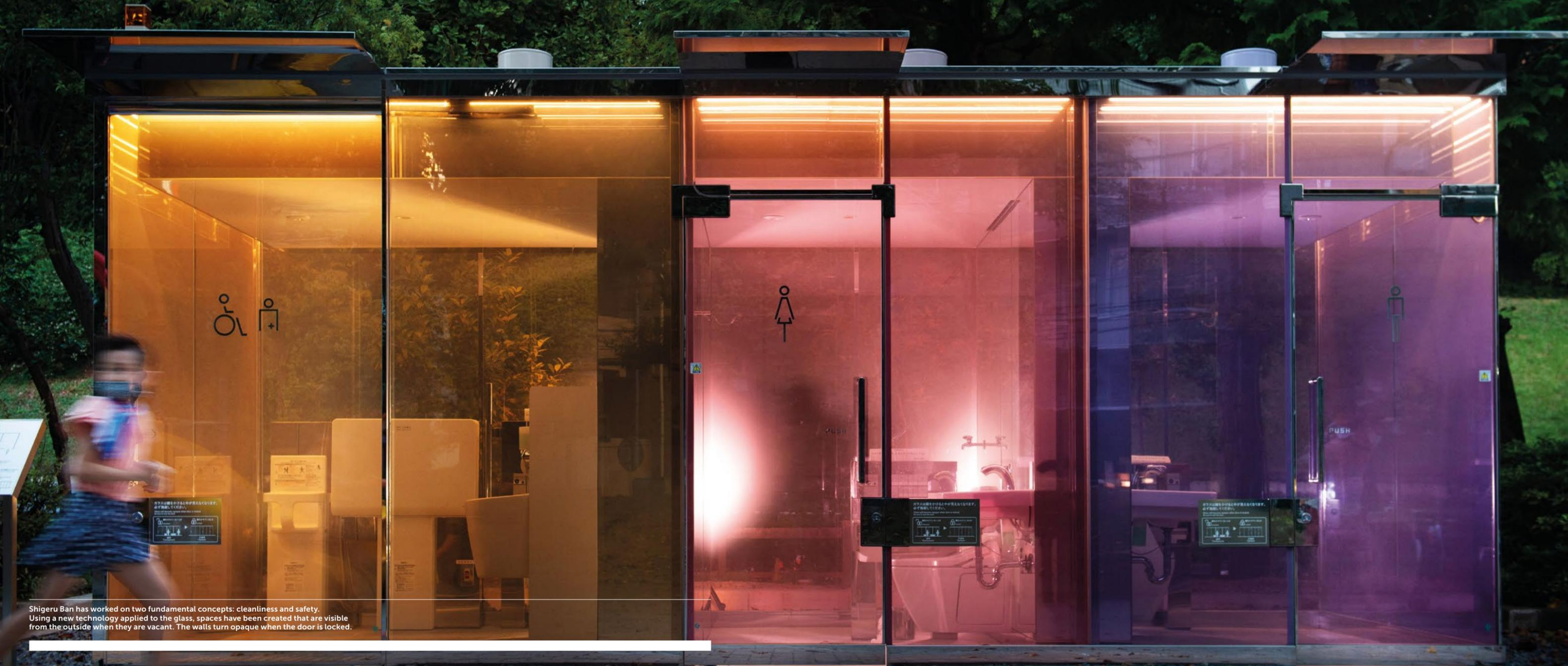
Shigeru Ban has worked on two fundamental concepts: cleanliness and safety. Using a new technology applied to the glass, spaces have been created that are visible from the outside when they are vacant. The walls turn opaque when the door is locked.
